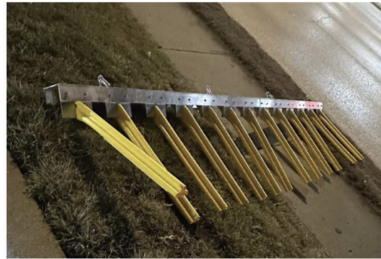
Photo Courtesy of Robert Ba | 11-foot-long piece of U-Channel aluminum that broke off and landed on a public sidewalk.
